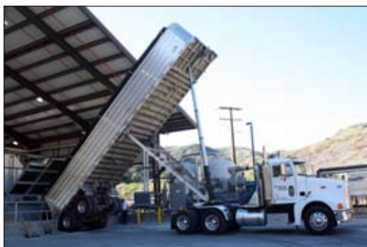
Biosolids from local wastewater treatment plants arrive at the facility by truck. For every four truckloads of wet biosolids, the drying process yields one truckload of dried material.
