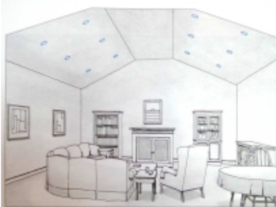
Figure 20 – A typical incandescent downlight-based living room design ( The Lighting Pattern Book for Homes )
